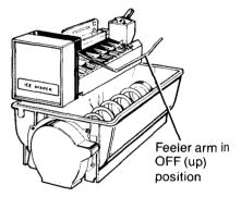
When water supply has been connected to icemaker, move feeler arm to ON (down) position.
